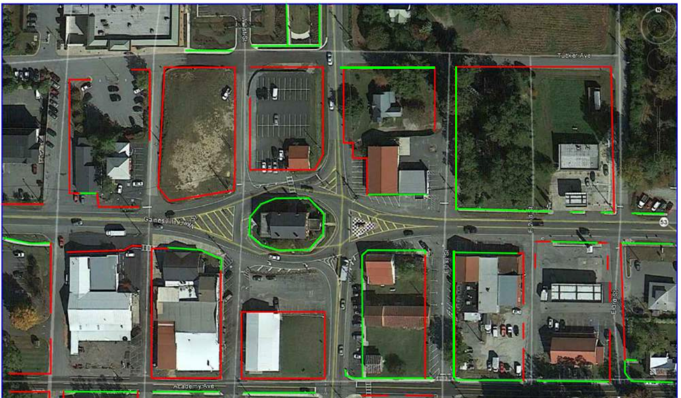
SIDEWALK INVENTORY. The map shown above highlights existing and needed sidewalks. Green areas indicate where sidewalks exist and red areas highlight where sidewalks are proposed to increase connectivity downtown.
